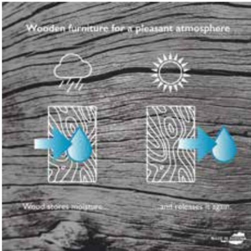
**Swelling:** If the air is humid, dry wood absorbs the humidity. This causes the cell walls to expand. The shape of the wood changes and becomes larger.
